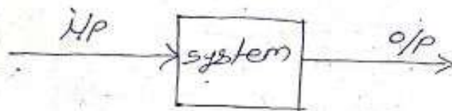
Block diagram of open loop control system
