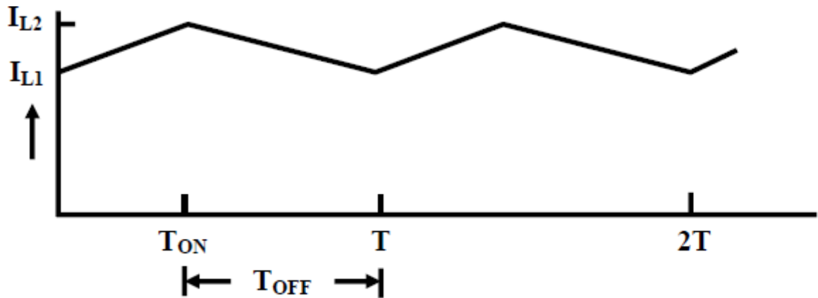
Fig. 17.3(b): Inductor current ( i_L ) waveform
