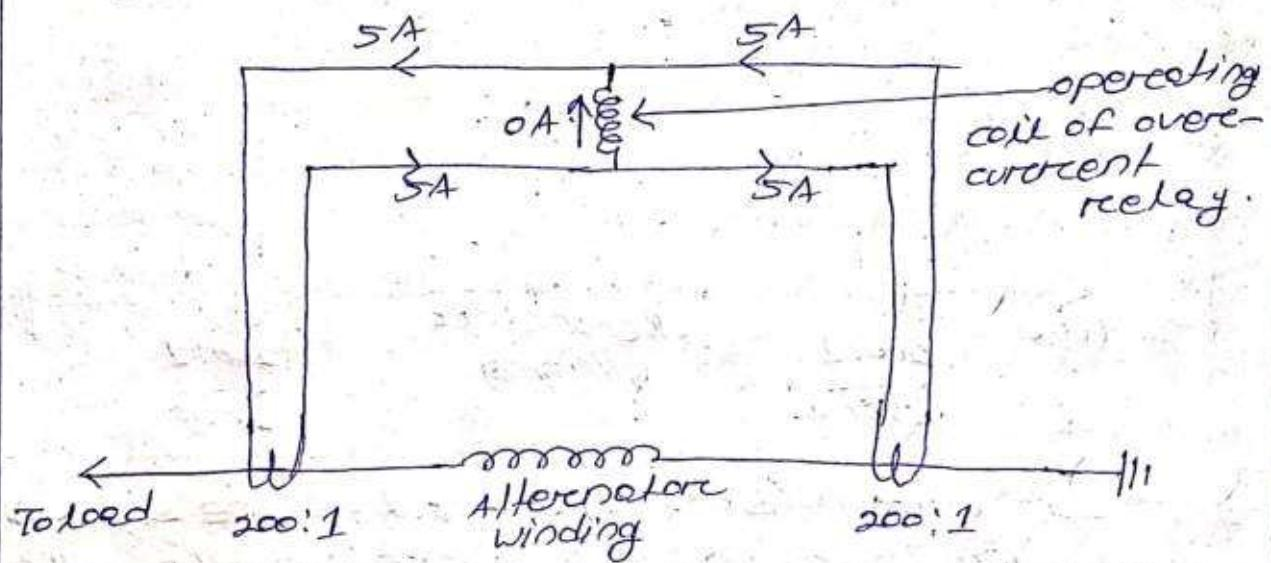
→ The secondary of CTs are connected in such a way that they carry the induced current in same direction.
