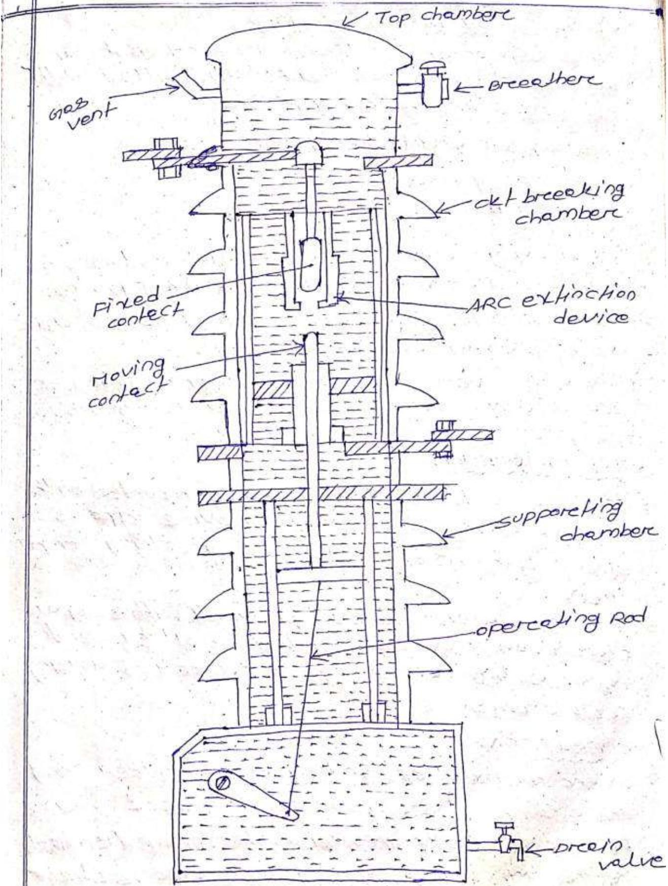
→ The oil inside the supporting chamber and the annular space formed between the porcelain insulation and Bakelite paper is employed for insulation purpose only.
