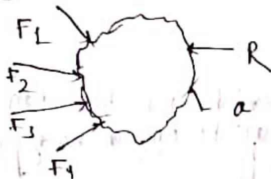
If a force of magnitude  $= R$  & is applied on the body along the line of action of the resultant in a direction opposite to the
