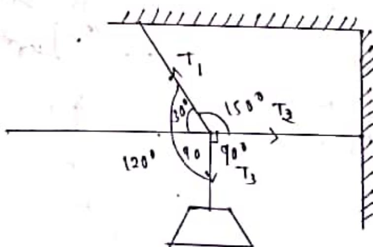
$T_1$  = Tension in the inclined string
