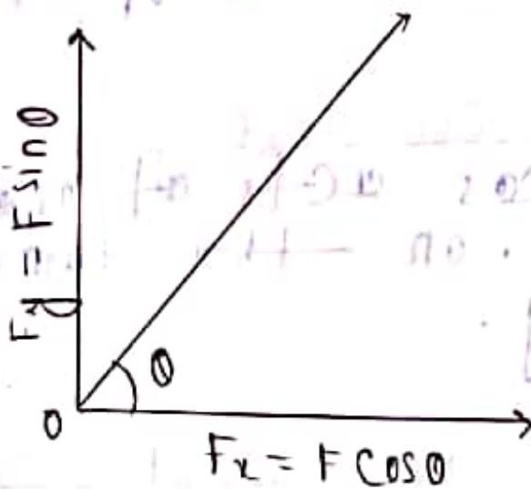
Let, a force 'F' is acting on a body at a point 'o' making angle 'θ' with horizontal.
