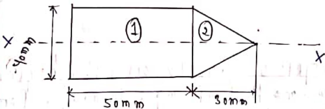
The composite section is symmetrical about x-x axis, hence the centroid is line.
