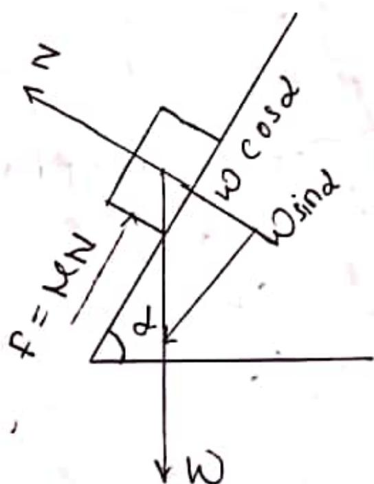
$\alpha$  = angle of inclination of the plane
