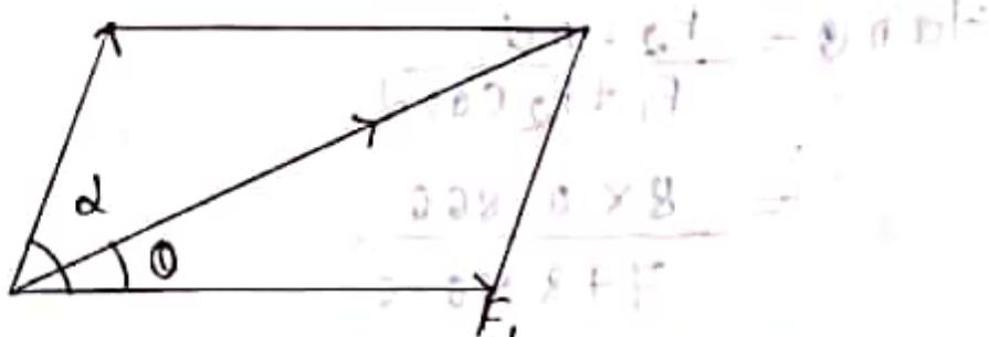
Let,  $F_1, F_2$  are two forces acting in the body the angle between two forces is  $\alpha$ .
