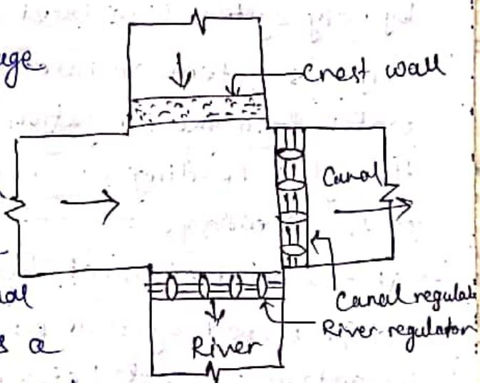
is closed while the cross regulator of the canal is kept open so that the canal flows without any interruption. During the flood, however, the drainage regulator is opened so that the flood discharge after spilling over the crest & mixing with the canal water, passes through it to the downstream of the drainage.
