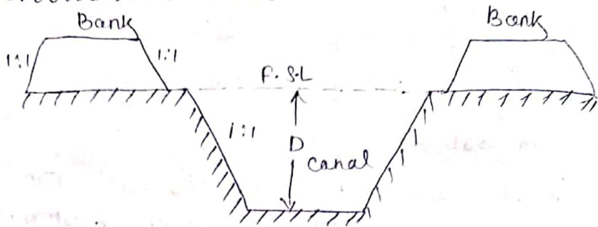
b) Canal in partially cutting & partially banking :-
