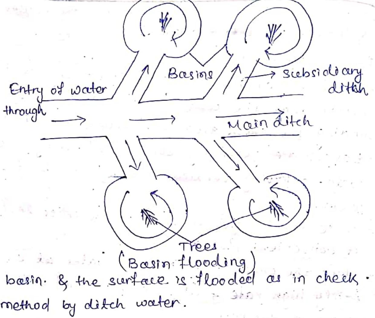
basin. & the surface is flooded as in check method by ditch water.
