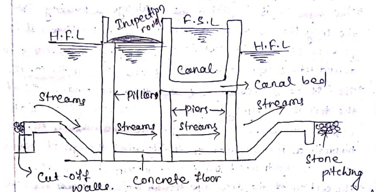
→ Here the sloping apron provided on both sides of the crossing. The apron may be constructed by cement concrete or stone pitching.
