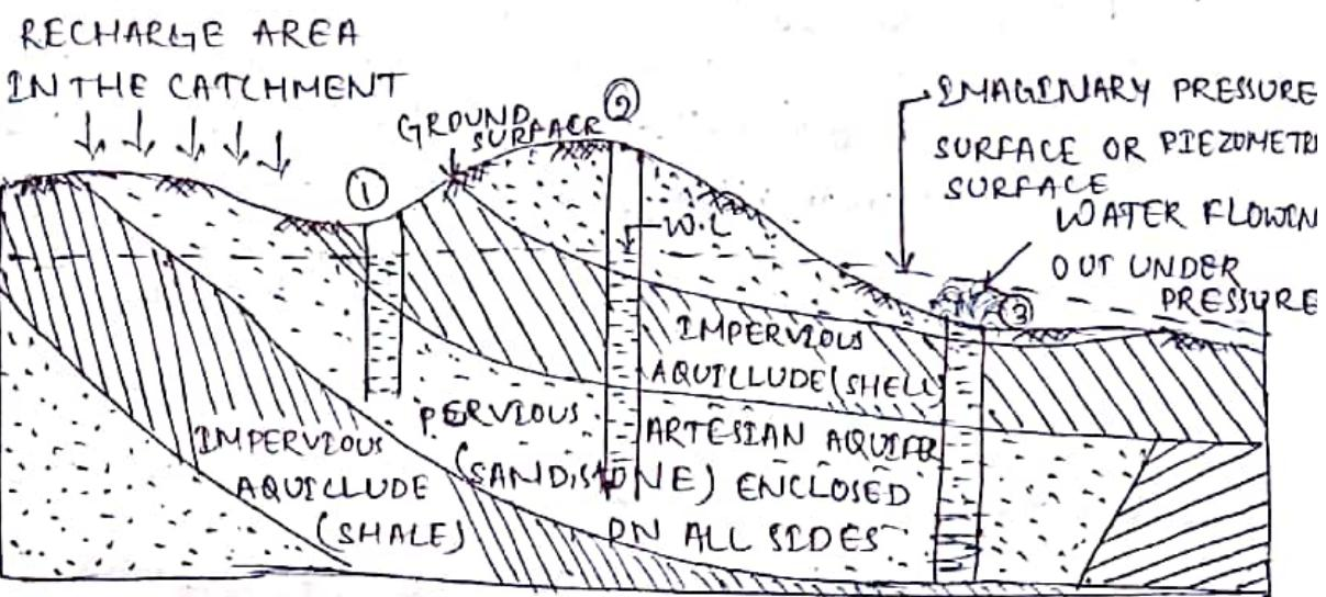
WELL NO 1 & 2 ARE NON-FLOWING ARTESIAN WELLS AND WELL 3 IS A FLOWING ARTESIAN WELL.
