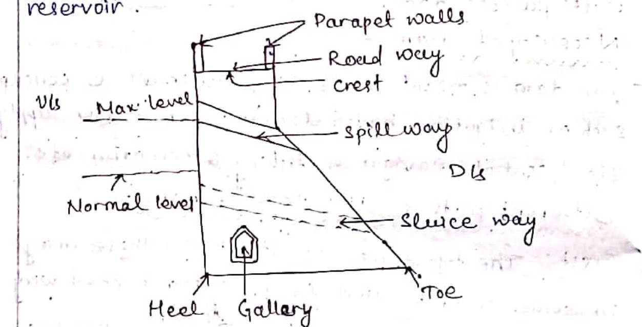
Gallery:- Level or gently sloping tunnel like passage (small room like space) at transverse or longitudinal within the dam with drain on floor for seepage water. These are generally provided for having space for drilling grout holes & drainage holes.
