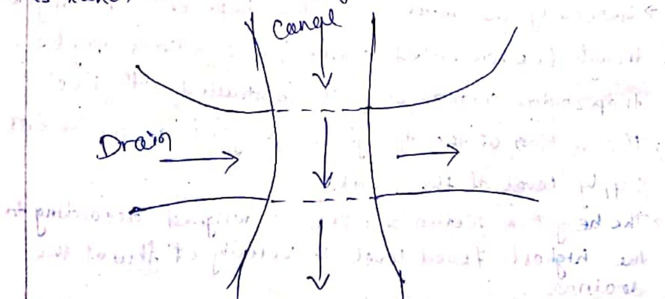
→ When the HFL of the drain is sufficiently below the bottom under gravity such type of structure is known as aqueduct.
