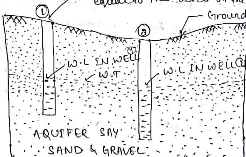
→ The ordinary gravity wells of 2 to 5 m diameter, which are constructed to gap water from the top most water bearing strata, i.e. from the unconfined aquifers, are known as unconfined or non-artesian wells.
